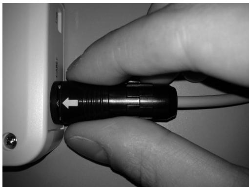
Grasp the locking collar of the ECG cable next to the arrow.
