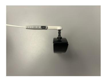
Screw the post all the way down, then attach your snap connector to the top.
