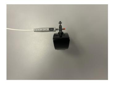
Unscrew the top screw to slide the banana plug into the hole in the post, then tighten the top screw to secure the plug.
